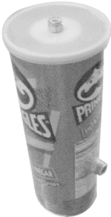
Figure 7-3. The completed antenna
